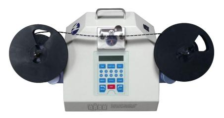
The SMD Reel Counting Equipment can count and count down SMD components packed in Reels, with speed and precision. It is an essential equipment for the management of SMD components.
