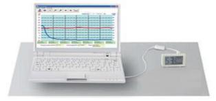
The humidity and temperature data can be downloaded and viewed on a computer using the USB connector and the thermo-hygrometer reader.
