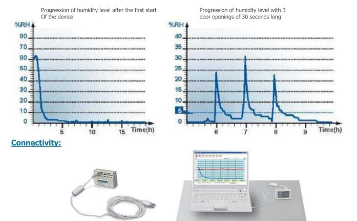
The humidity and temperature data can be downloaded and viewed on a computer using the USB connector and the thermo-hygrometer reader.
