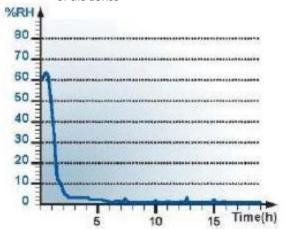
Progression of humidity level with 3 door openings of 30 seconds long
