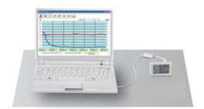
The humidity and temperature data can be downloaded and viewed on a computer using the USB connector and the thermo-hygrometer reader.
